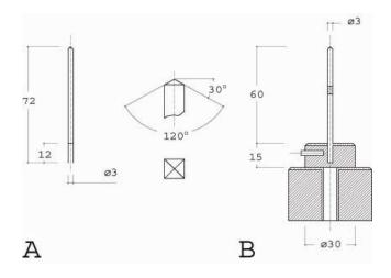
Figure A.1. High speed dynamometer for test of cloth resistance to perforation
