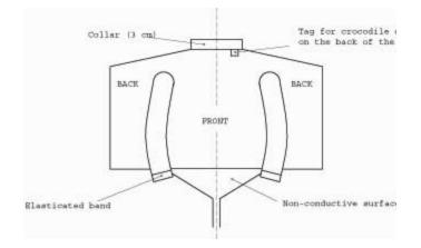
Figure 15. Electric saber conductive jacket
