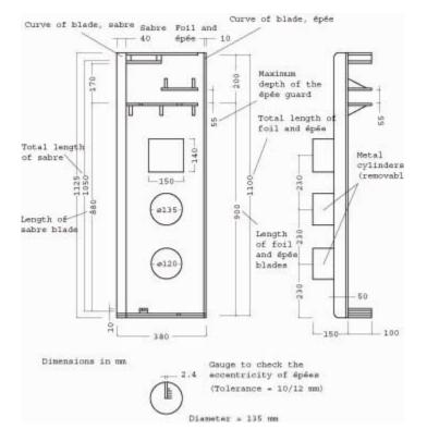
Figure 16. Gauge for checking weapons
