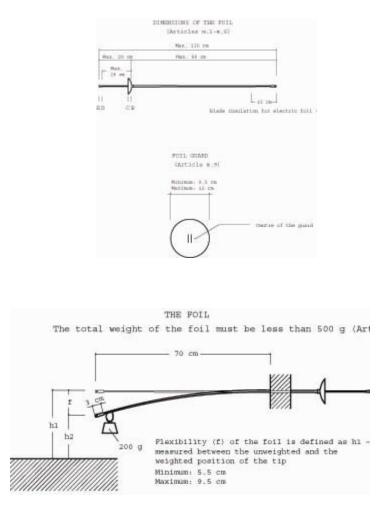
Figure 8. Foil dimensions and flexibility
