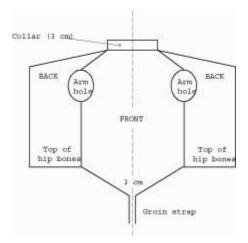
Figure 14. Foil: conductive jacket
