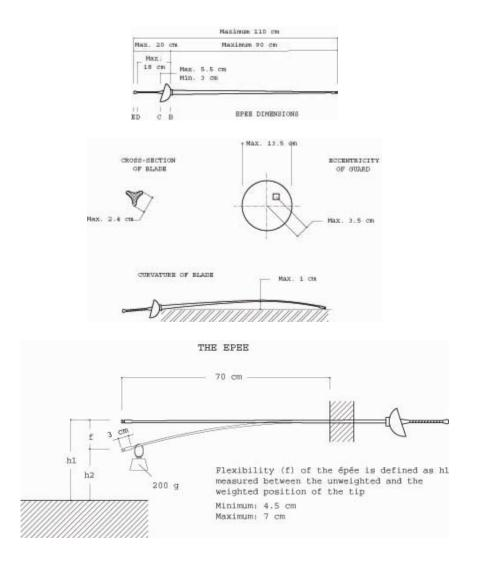
Figure 9. Epee dimensions and flexibility
