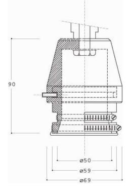
Figure A.3. Fixing device for test of cloth resistance to perforation
